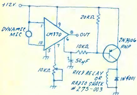
IC. The level at which the circuit trips is set by the 10K pot connected to pin 7 of the IC. When activated, the relay is switched on. How the contacts are wired is left to you. By the way, the LM370 seems to be the IC of choice for voice actuated circuits.
