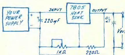
tor IC. Normally, the 7805 is a fixed voltage regulator producing five volts output. But by adding a 220 ohm fixed resistor and a 1K pot, the IC is tricked into producing a variable output determined by the control setting. One drawback to this circuit is that it can't get down to voltages much below five volts. If you need lower voltages, you can substitute an LM317, an excellent regulator, but not currently available at Radio Shack.
