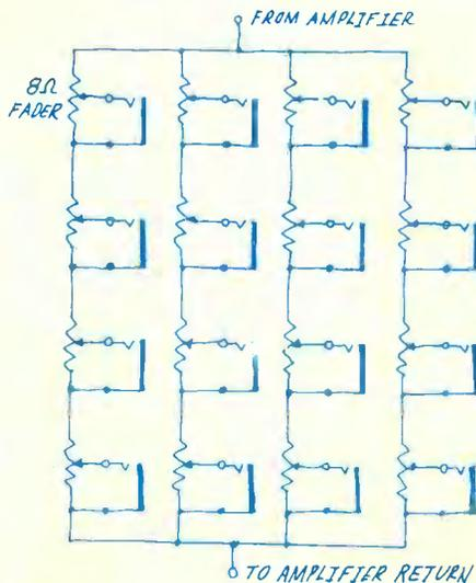
faders in series. The net impedance of the circuit is eight ohms, an ideal load for your Fisher. One nice feature of this simple circuit
