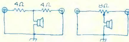
good advice because it is possible for one channel to drive the other. You can get around the problem by connecting the circuit so that each channel still sees a reasonable load. You can use a pair of four ohm resistors, or an eight ohm control between the two outputs, with the speaker connected from the junction or wiper to ground.
